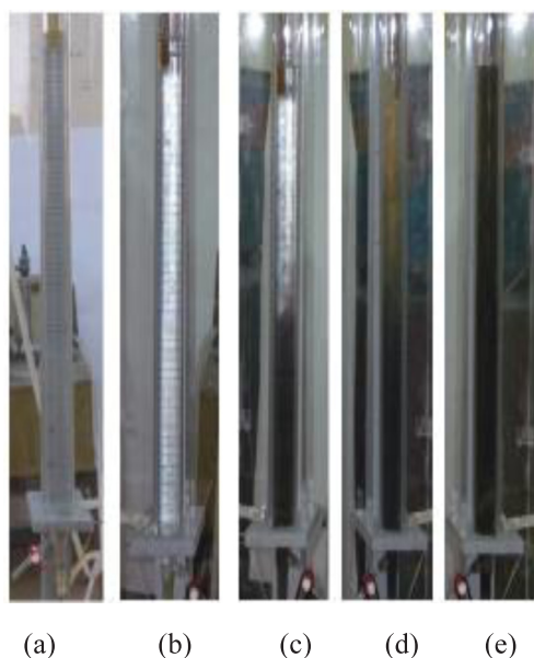
Figure 3. Color change of aqueous medium at high voltage electrochemical reaction times of Ag electrode from (a) 0 min to (b) 5 min, (c) 10 min, (d) 20 min and (e) 30 min.
